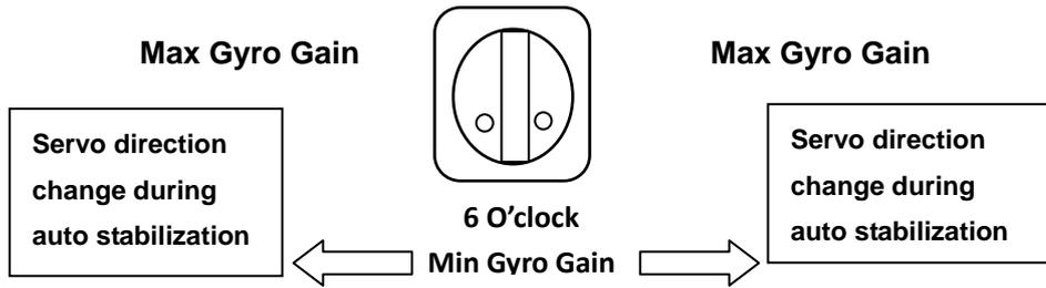
(2) Gyro Gain: The further away from Centre (6 O'clock) the higher the Gyro gain (sensitivity). Too low gain result is poor auto stabilization, too high gain will cause oscillations of the aircraft. You need to adjust the gain setting based on the requirement of your aircraft.
